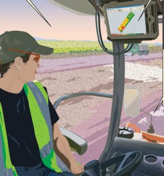
On-location infrared camera detects thermal segregation in freshly placed asphalt mat; image shows range of 154 deg F (green) to 206 deg F (red), indicating
