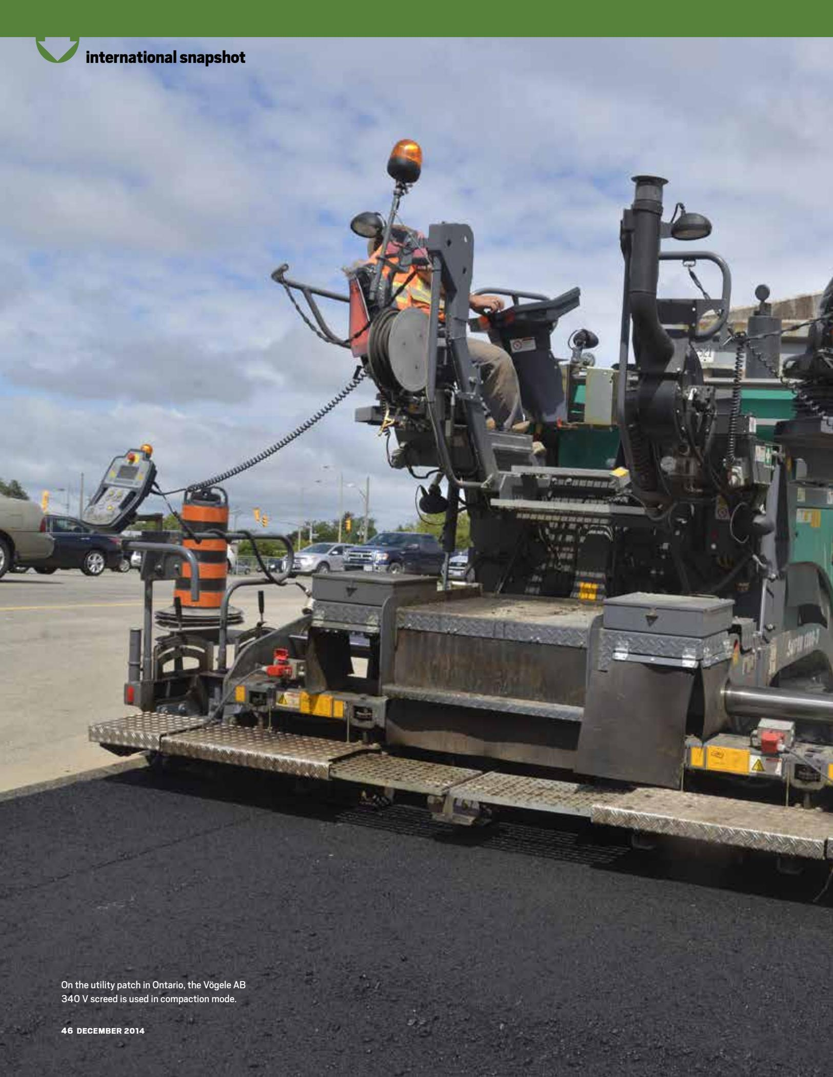
On the utility patch in Ontario, the Vögele AB 340 V screed is used in compaction mode.
