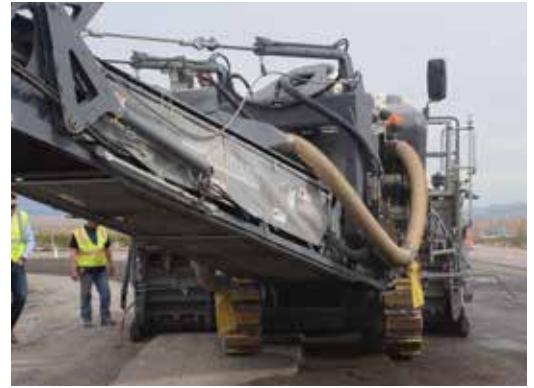
LEFT: "The grade control has seven points of control, and what we really like is that it's holding the 2 percent crossfall really well," Jason Torres said. RIGHT: "When we are dumping on the shoulders, were getting a 25 percent improvement..." — Jason Torrese. BELOW: Las Vegas Paving uses the W 250i full-lane cold mill from Wirtgen to mill 27 miles in both directions on I-15 north of Las Vegas. The machine is Wirtgen's biggest cold mill and generates a total of 991 horsepower with two engines engaged while meeting Tier 4 Interim emissions regulations.
