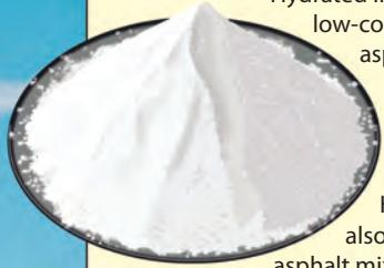
Hydrated lime is a low-cost, near-generic asphalt modifier that performs powerful anti-stripping functions. Hydrated lime also makes an asphalt mix stiffer, tougher, and resistant to rutting, and may have other attributes as well
