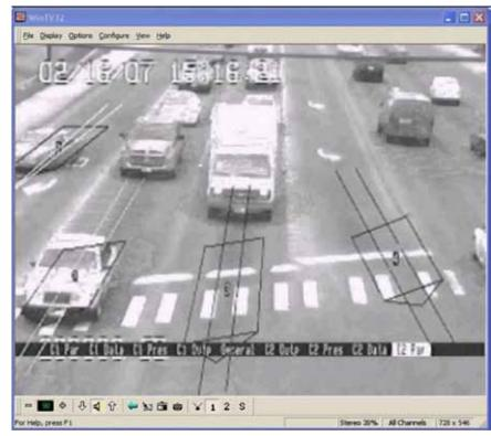
■ Video Image Processors (VIPs) have been increasingly deployed for intersection signal control over the past decade. A VIP can support up to 24 virtual loops, but normally less than half of the virtual loops are used. By properly configuring the spare virtual loops and analyzing the loop measurements, intersection performance can be monitored in real time.
