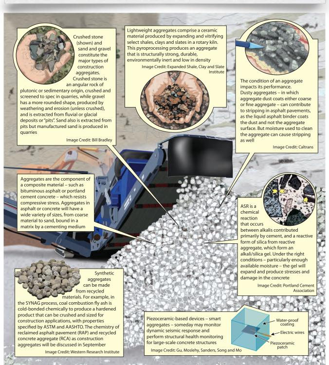
primarily by cement, and a reactive form of silica from reactive aggregate, which form an alkali/silica gel. Under the right conditions – particularly enough available moisture – the gel will expand and produce stresses and damage in the concrete.
