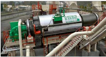
introducing water at high rates through one nozzle, so we went to multiple nozzles," Brock says. "The first unit we came out with had 10 nozzles, but we have adjusted the size and number of the openings, and done machining to get the system to the right point where it will blend asphalt and water properly." Today's units have six nozzles.
