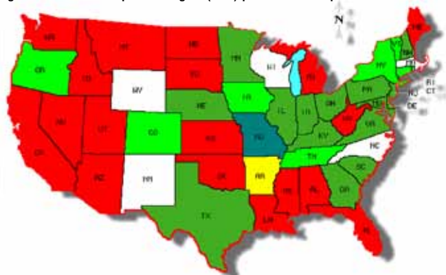
A May 2011 survey by RAP Expert Task Group found maximum allowable percentages of reclaimed asphalt shingles (RAS) permitted in asphalt mixes.
