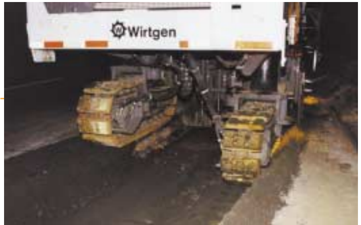
Independent suspension of 2100 DC works well with Combo Cutter
