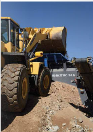
LEFT The loader feeds the MC 110 Zi EVO. ABOVE While the Domres managers are pleased with the elliptical motion of the pre-screen on the machine, Kleemann offers both vibrating grizzly (G) and independent pre-screen (L) models in modern configurations for 2014. "We want to offer a machine with the same features as competing manufacturers, while presenting a different model that may cost a little more, but provides the enhanced productivity of the independent pre-screen," Kleemann technical service manager Kelly Graves said. Both models are Tier 4 Final emissions-compliant. The new MC 110 Ri EVO has a vibratory feeder with integrated grizzly, while the value-added MC 110 Zi EVO incorporates a vibrating feeder with an independent, double-deck, heavy-duty pre-screen.
