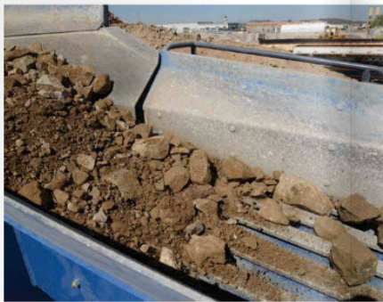
LEFT The loader feeds the MC 110 Zi EVO. ABOVE While the Domres managers are pleased with the elliptical motion of the pre-screen on the machine, Kleemann offers both vibrating grizzly (G) and independent pre-screen (L) models in modern configurations for 2014. "We want to offer a machine with the same features as competing manufacturers, while presenting a different model that may cost a little more, but provides the enhanced productivity of the independent pre-screen," Kleemann technical service manager Kelly Graves said. Both models are Tier 4 Final emissions-compliant. The new MC 110 Ri EVO has a vibratory feeder with integrated grizzly, while the value-added MC 110 Zi EVO incorporates a vibrating feeder with an independent, double-deck, heavy-duty pre-screen.
