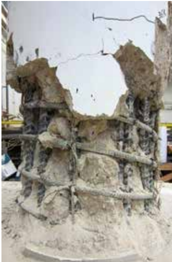
Seismically damaged column repair procedure with the hybrid confining jacket. From left to right, damaged column; patched column with repair grout; sheet metal wrapping; prestressing strands application
