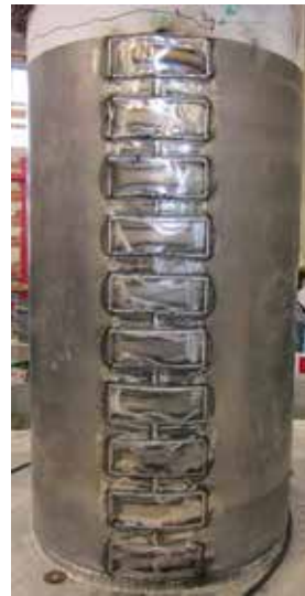
Seismically damaged column repair procedure with the hybrid confining jacket. From left to right, damaged column; patched column with repair grout; sheet metal wrapping; prestressing strands application
