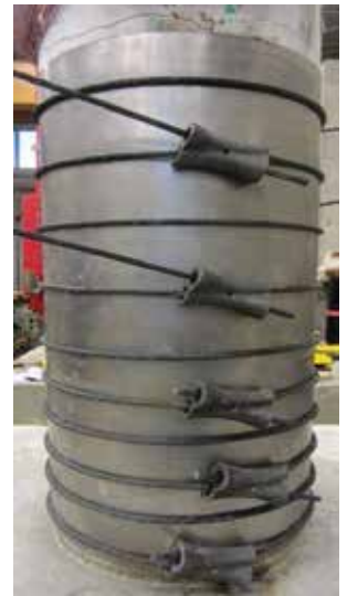
Seismically damaged column repair procedure with the hybrid confining jacket. From left to right, damaged column; patched column with repair grout; sheet metal wrapping; prestressing strands application
