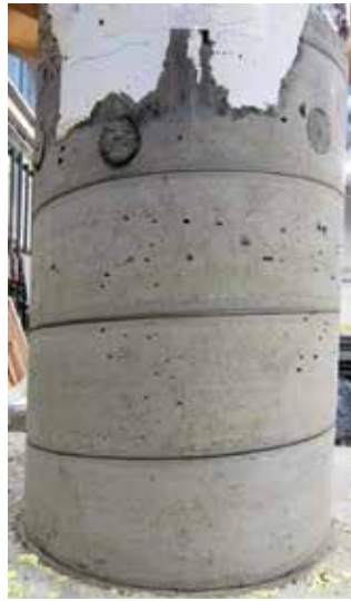
Seismically damaged column repair procedure with the hybrid confining jacket. From left to right, damaged column; patched column with repair grout; sheet metal wrapping; prestressing strands application
