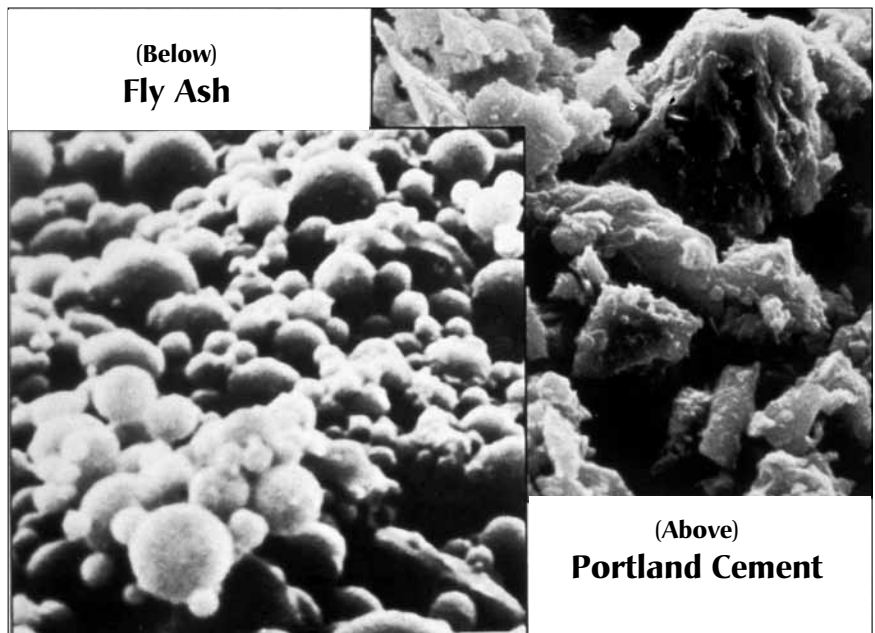
▲ Relative appearance of fly ash and portland cement in micrographs.
