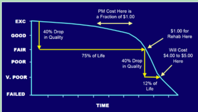
▲ The essence of pavement preservation is the application of the right treatment, to the right pavement, at the right time to save or delay future expenditures. Photo courtesy of FP 2
