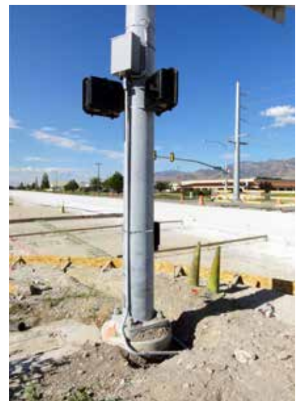
Utah portland cement concrete pavement albedo experiment site instrumentation: left, temperature sensors for monitoring concrete pavement; center, sensor cables in PVC pipe; and right, utility box mounted on signal pole. IMAGES: Guthrie, Waters and Knighton.
