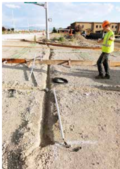
Utah portland cement concrete pavement albedo experiment site instrumentation: left, temperature sensors for monitoring concrete pavement; center, sensor cables in PVC pipe; and right, utility box mounted on signal pole. IMAGES: Guthrie, Waters and Knighton.
