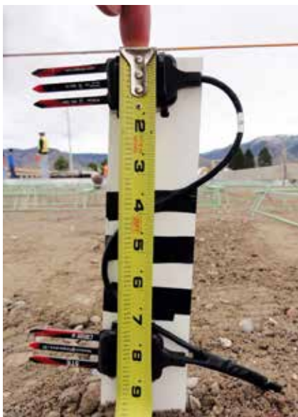
Utah portland cement concrete pavement albedo experiment site instrumentation: left, temperature sensors for monitoring concrete pavement; center, sensor cables in PVC pipe; and right, utility box mounted on signal pole. IMAGES: Guthrie, Waters and Knighton.
