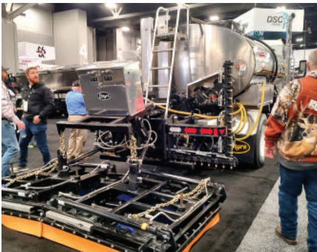
In a large stand, E.D. Etnyre & Co. displayed its scrub seal applicator attached to emulsion distributor truck https://etnyre.com/
