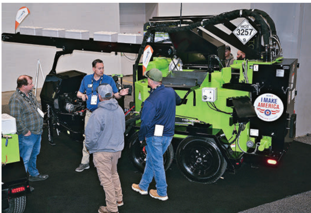
Cimline showed its versatile M-4 melter applicator for joint and crack sealing www.cimline.com
